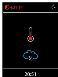
**When the sauna is switch on** - the thermometer symbol starts to pulse red during the heating up time, after this it will continuously light in red.
